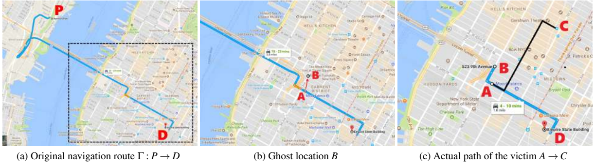
Figure 3: An attack example: the victim’s original navigation route is P \rightarrow D ; At location A , the spoofer sets the GPS to a ghost location B which forces the navigation system to generate a new route B \rightarrow D . Following the turn-by-turn navigation, the victim actually travels from A to C in the physical world.
