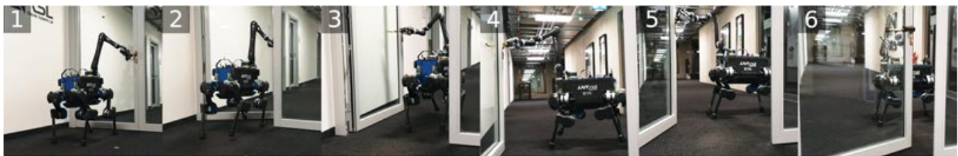
Fig. 10. Commanding a contact force task instead of a motion task for the gripper allows the robot to open a spring-loaded door without requiring exact knowledge of the door kinematics. Integration of this task in the whole-body controller combined with the COM-based locomotion controller enable the robot to simultaneously perform a trotting gait to pass through the door.
