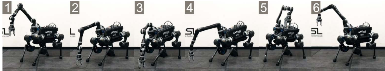
Fig. 8. By setting up an angular velocity reference task for the floating base, the robot adapts its posture to increase the kinematic reach of the gripper. The figure shows the torso adaptation for different end-effector locations.
