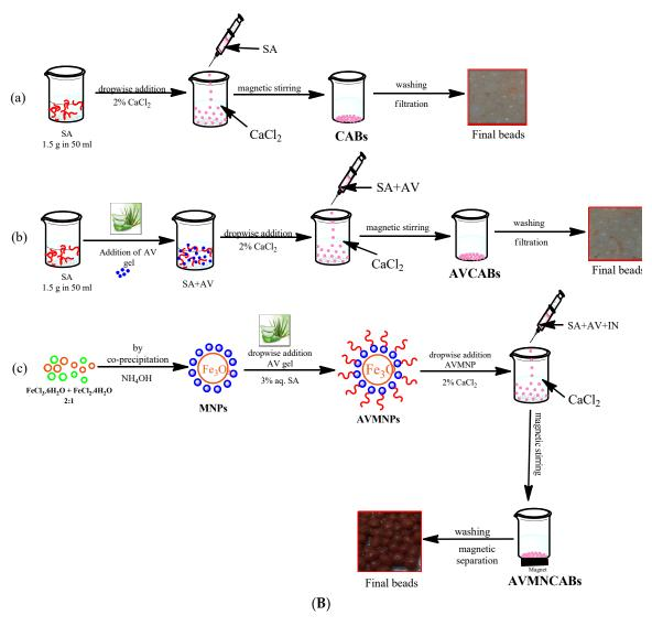
**Figure 1.** (**A**) Images of the (**a**) CABs, (**b**) AVCABs and (**c**) AVMNCABs gel beads (approximate size of beads: 2–3 mm); (**B**) Synthesis of (**a**) CABs, (**b**) AVCABs, and (**c**) AVMNCABs gel beads.
