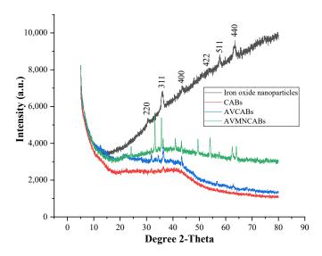
**Figure 3.** XRD patterns of iron oxide ( $Fe_3O_4$ ) nanoparticles, CABs, AVCABs, and AVMNCABs, with the characteristic peaks of  $Fe_3O_4$  identified.
