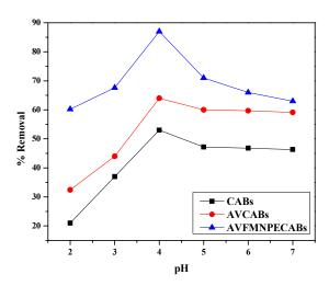
**Figure 8.** pH effect on Cu(II) removal for an initial concentration of 10  $\mu$ g mL<sup>-1</sup>; 0.2 g adsorbent; 1 h.
