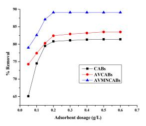
**Figure 10.** Variation of the removal of Cu(II) with adsorbent dose (10  $\mu$ g mL<sup>-1</sup> Cu(II), 1 h, 30 °C, pH 4).
