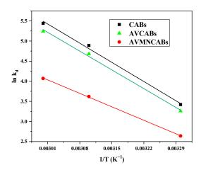
**Figure 15.** Van't Hoff's plot for Cu(II) adsorption.
