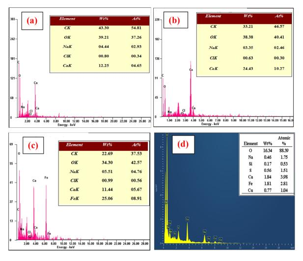
**Figure 7.** EDX spectra of **(a)** CABs, **(b)** AVCABs, and **(c)** AVMNCABs before adsorption; and **(d)** AVMNCABs after adsorption.
