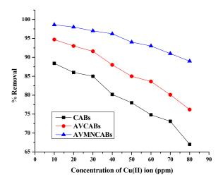
**Figure 12.** Effect of the initial Cu(II) concentration on the adsorption (0.2 g adsorbent, 120 min, 30  $^{\circ}$ C, pH 4).
