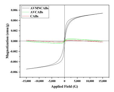
**Figure 5.** Vibrating sample magnetization (VSM) of CABs, AVCABs, and AVMNCABs (at room temperature).
