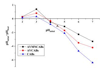
Figure 9. Point of zero charge (pH<sub>pzc</sub>) of AVMNCABs, AVCABs, and CABs.
