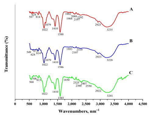
Figure 4. FTIR spectra of (A) CABs, (B) AVCABs, and (C) AVMNCABs before adsorption.
