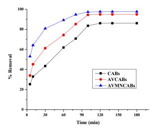
Figure 11. Effect of time on the removal of Cu(II) (10  $\mu$ g mL<sup>-1</sup> Cu(II), 0.2 g adsorbent; 30 °C, pH 4).
