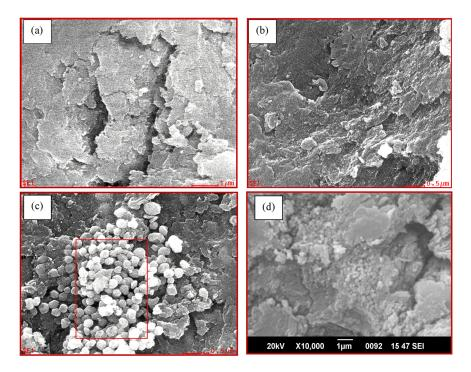
**Figure 6.** SEM images of **(a)** CABs, **(b)** AVCABs, and **(c)** AVMNCABs before adsorption and **(d)** AVMNCABs after adsorption.
