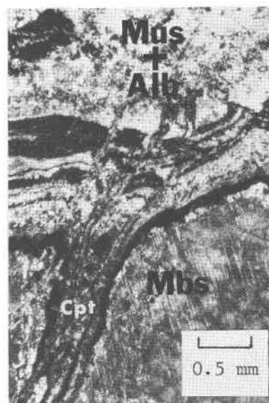
Fig. 9. Photomicrograph showing a rim of carbonate-apatite (Cpt) surrounding primary montebrasite (Mbs). The fine-grained assemblage above the apatite is an intergrowth of muscovite (Mus) + albite (Alb) after spodumene. As illustrated in this sample from the Midnight Owl pegmatite, wherever spodumene occurs with montebrasite (or near lithiophilite), the spodumene is invariably more extensively altered than the phosphate. Crossed polars.
