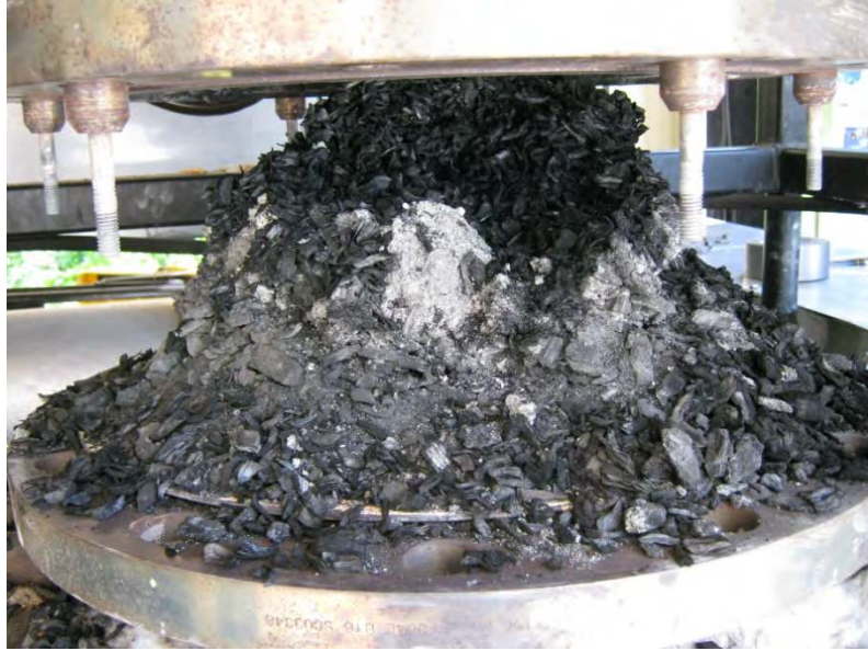
Figure 9-8: Gasifier opened at seam 10cm above the grate
