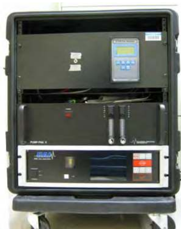
Figure 9-14: Gas analyzer train used during experiments. HiTech K1550 top right, California Analytical ZRE bottom, California Analytical Pump Pack II middle
