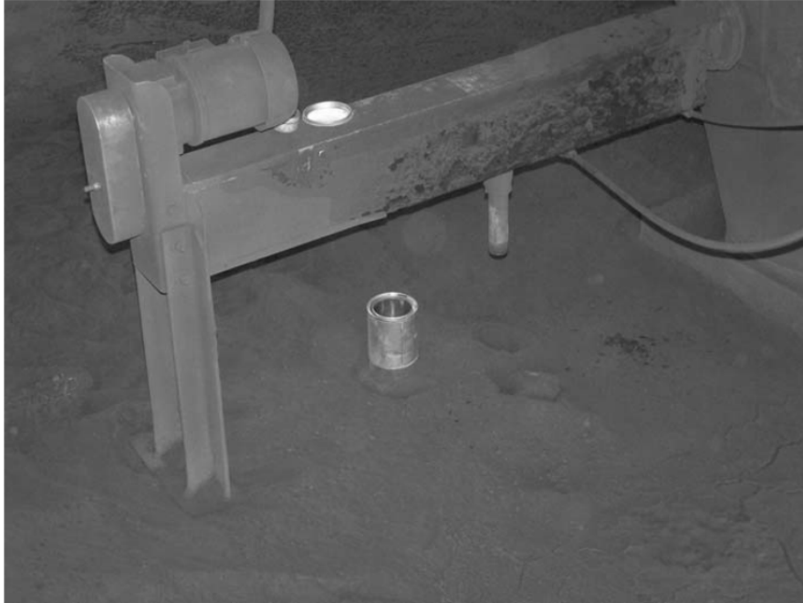
Figure 4-11: Automated Plunger System
