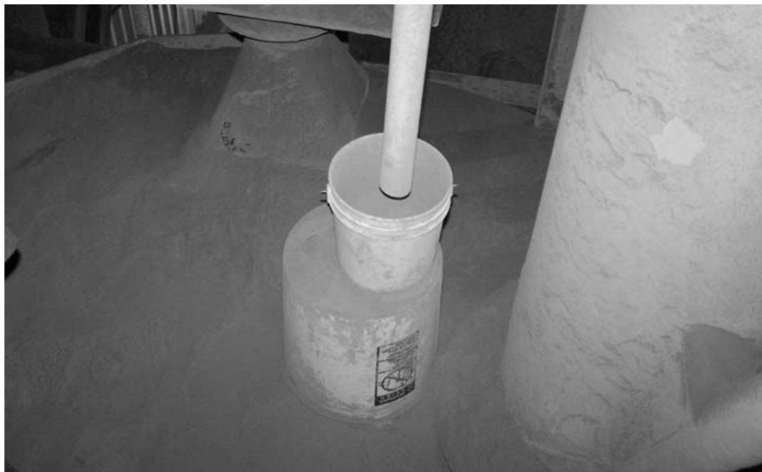
Figure 4-13: Portland Cement Sampling Point
