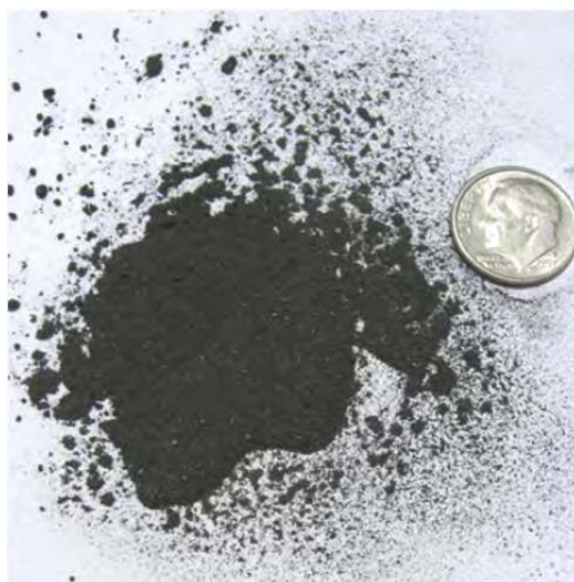
Figure 10-30: Char from inside and just after the heat exchanger, labeled 'HEX'
