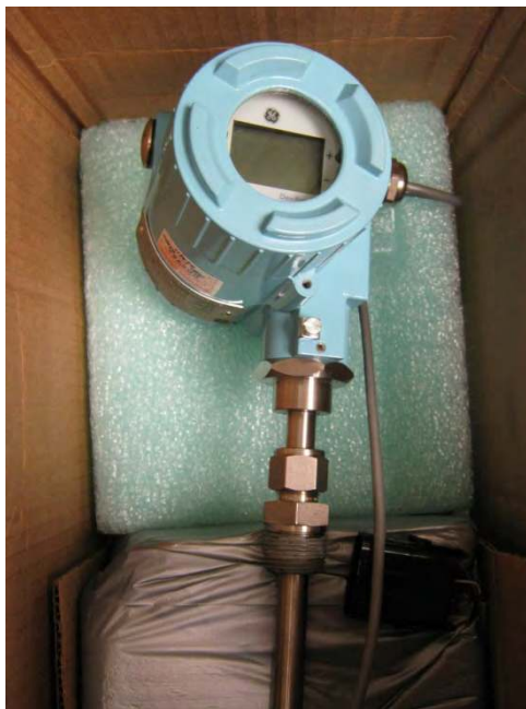
Figure 9-15: DewPro MMR101 used in contaminant quantification experiments, measures % volume moisture
