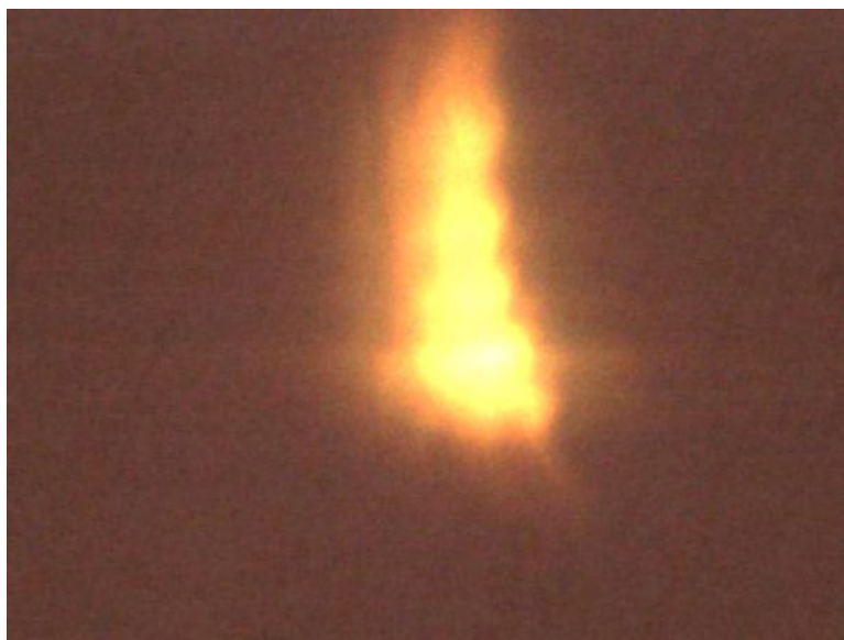
Figure 2-3: Wood at 900 °C in air (100 micrometer nominal particle)
