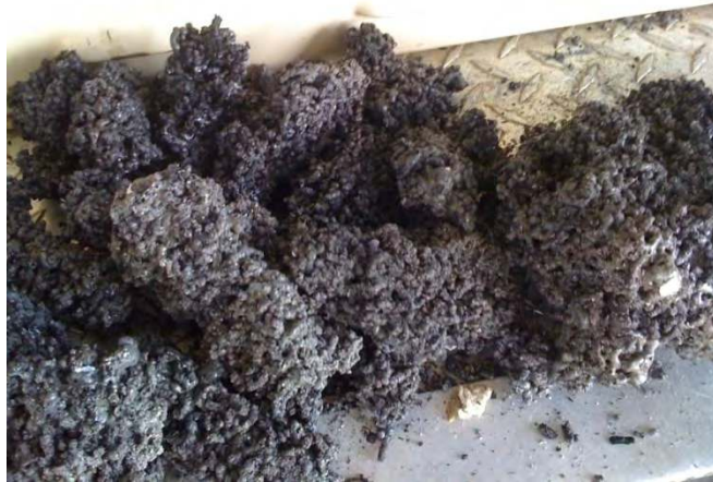
Figure 10-19: Poultry litter pellet clinkers from 40% pellet run
