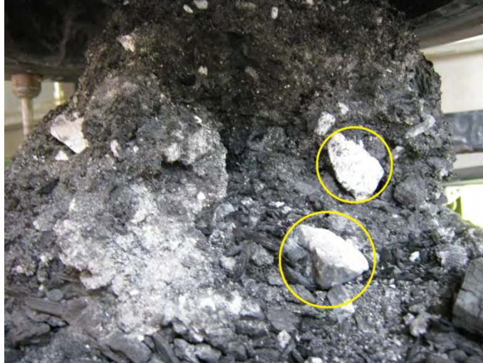
Figure 10-26: Ash mound found when gasifier is opened at seam above the grate, white deposits circled
