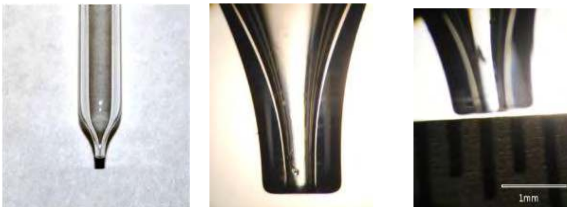
Figure 2-15: Glass nozzles for the piezoelectric drop generator
