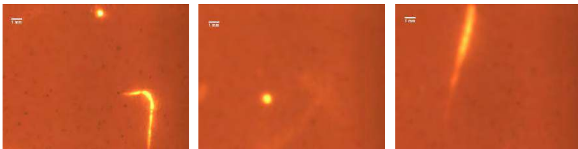
Figure 2-5: Images of switch grass particles undergoing combustion in air at 900 °C
