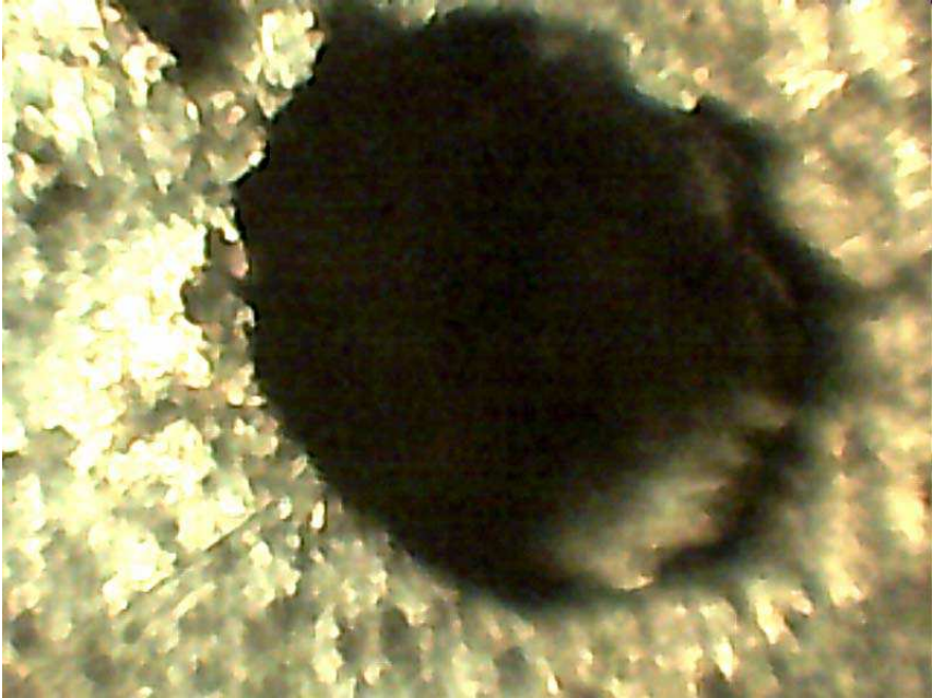
Fig. 5. A Blow hole defect in an aluminum casting at 100× magnification
