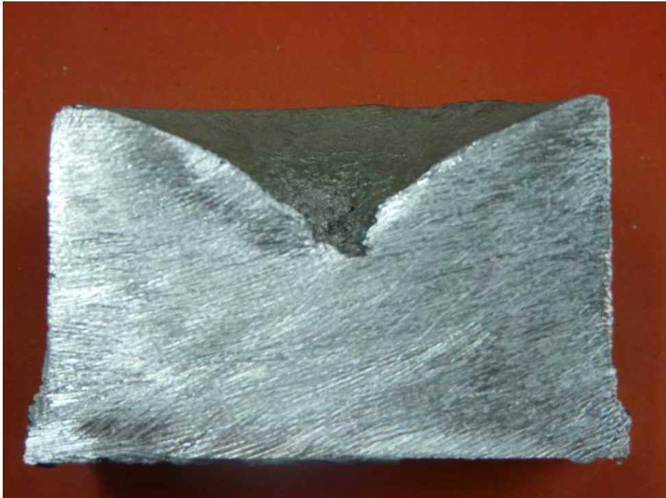
Fig. 7. Typical appearance of volumetric shrinkage defect in an aluminium section
