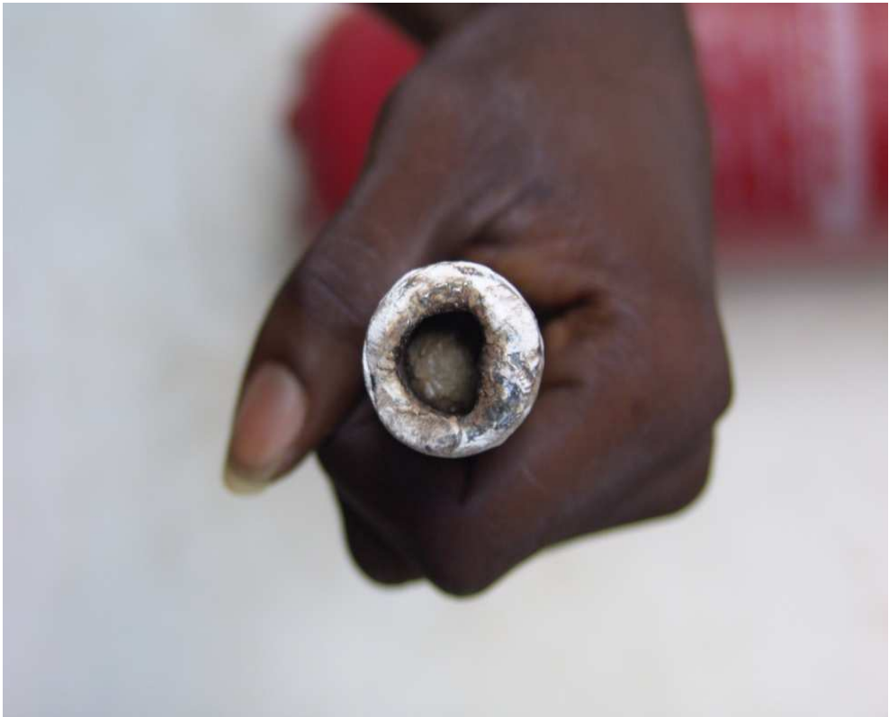
Fig. 12. Premature solidification of melt inside the sprue due to inadequate pre-heat
