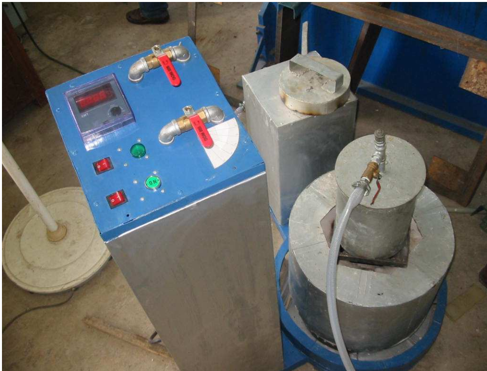
Fig. 13. A low-cost machine for countergravity casting
