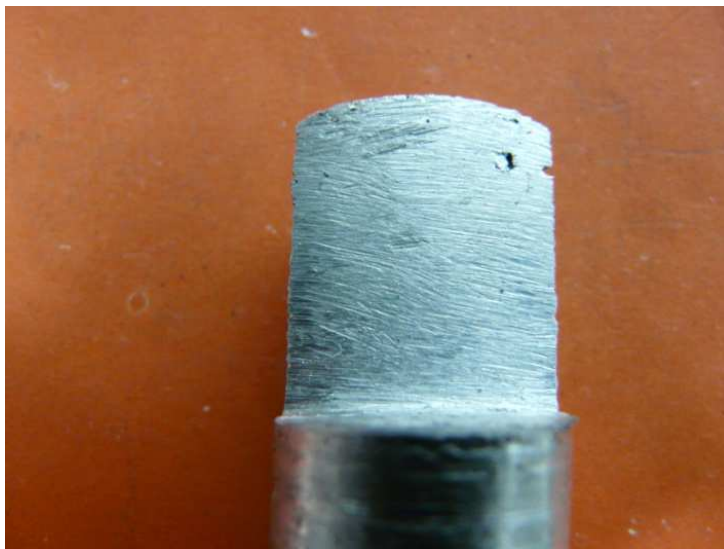
Fig. 8. Cross-section of a countergravity cast rod showing the absence of volumetric shrinkage defect as evident from the convex meniscus at the top of the rod
