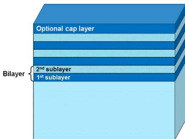
FIG. 1. (Color online) Schematic representation of a typical nanolaminate structure with three bilayers and a cap layer.
