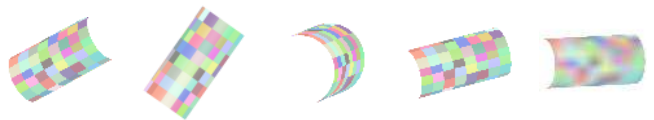
Fig. 3. Applying a 8 \times 16 texture over a cylinder impostor, using a prism mapping M_c . For illustration purposes, bilinear interpolation is disabled, except in the last image, and random color values are assigned to texels. Duplicated texels are assigned to the same color.
