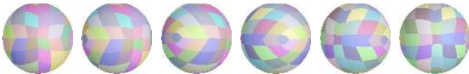
Fig. 2. Applying a small 2D texture map over a sphere impostor, using a 10 \times 10 octahedron mapping M_{s2} . In order to show the behavior of M_{s2} the virtual sphere (impostor) is rotated from left to right by 180^\circ . For illustration purposes bilinear interpolation is disabled and random values are assigned to texels, so that they are clearly visible. Duplicated texels are assigned to the same color (see later). Refer to fig. 6 to see the used 2D texture.
