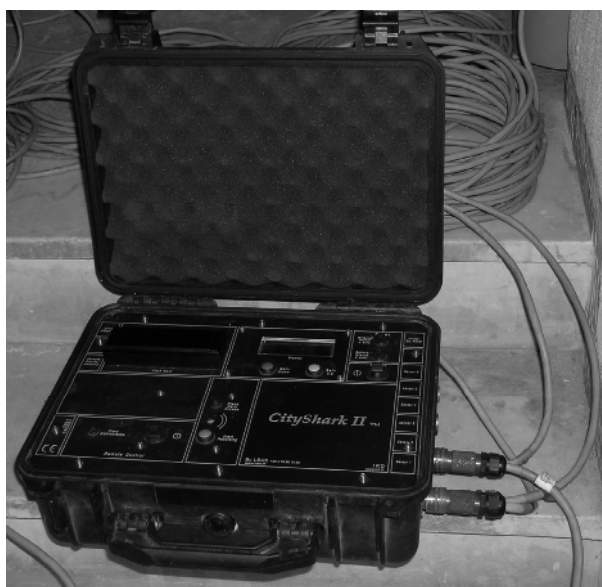
Figure 1. View of a CityShark II-6 station.
