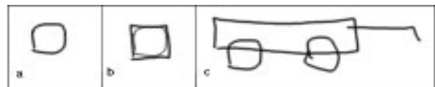
Figure 5. (a) A blob shape matches both Circle and Box. (b) The user resolves it as a Box by drawing over it, or (c) the Napkin resolves it as a Circle from its position in a configuration.
