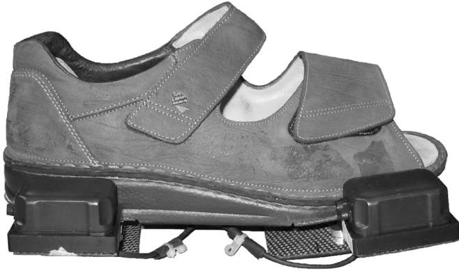
Fig. 1. Instrumented shoe with force transducers, and inertial sensors.
