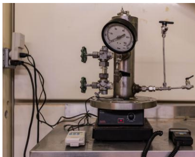
Figure 01 Small thermostated VLE cell
