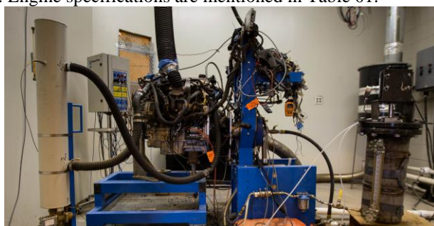
Figure 03 SuperFlow 902 engine dynamometer with Eco-Tec LE5 2.4L engine
