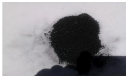
Fig. 1: Bamboo charcoal of \leq 600\mu\text{m} particle sizes
