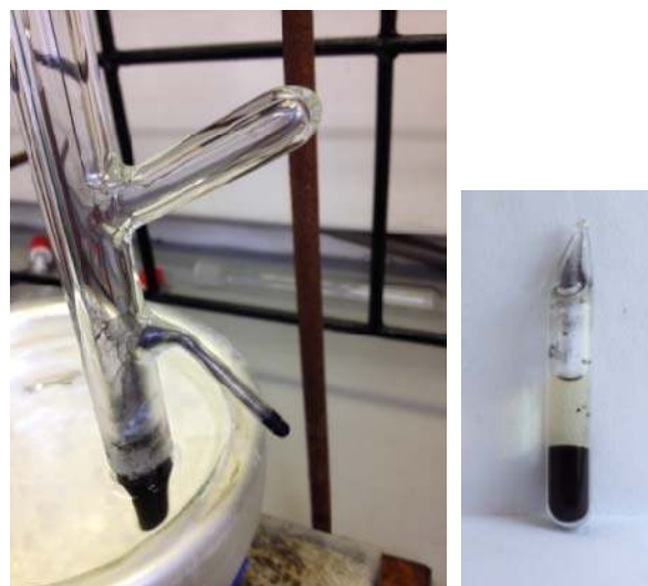
Figure S9. Apparatus for handling the ammonia-rich solid in liquid ammonia. The ratio of the glass wall thickness to the overall diameter must be chosen to ensure that the autogenous pressure of ammonia does not rupture the tube. E.g. 18 mm o.d. × 4mm wall for the reaction tube shown left (similar to that used on I12) or 5mm o.d. × 1 mm wall for the spur sealed off for the magnetometry measurements (right). Refer to the glass supplier's data and use a professional glassblower to construct the apparatus.
