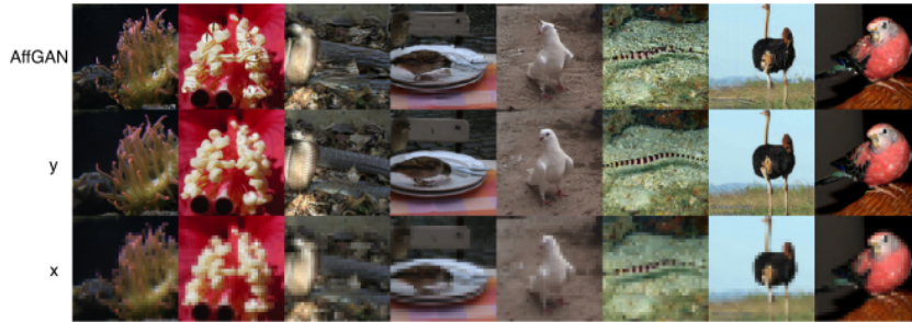
Figure 5: 4\times SR from 32\times 32 to 128\times 128 using AffGAN on the ImageNET. AffGAN outputs (top row), true HR images y (middle row), model input x (bottom row). Generally the AffGAN produces plausible outputs which are however still easily distinguishable from true images. Interestingly the snake depicted in the third column is super resolved into water which is obviously wrong but still a very plausible image considering the LR input image.
