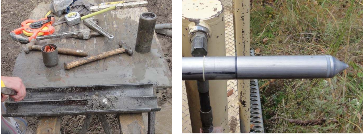
Figure 2.1. Photographs of a) the California split spoon sampler used for the SPT (Coffman 2011a) and b) the cone used for the CPT (as used during the geotechnical investigation at the MATS, TATS, and SSATS) by Coffman (2011b).
