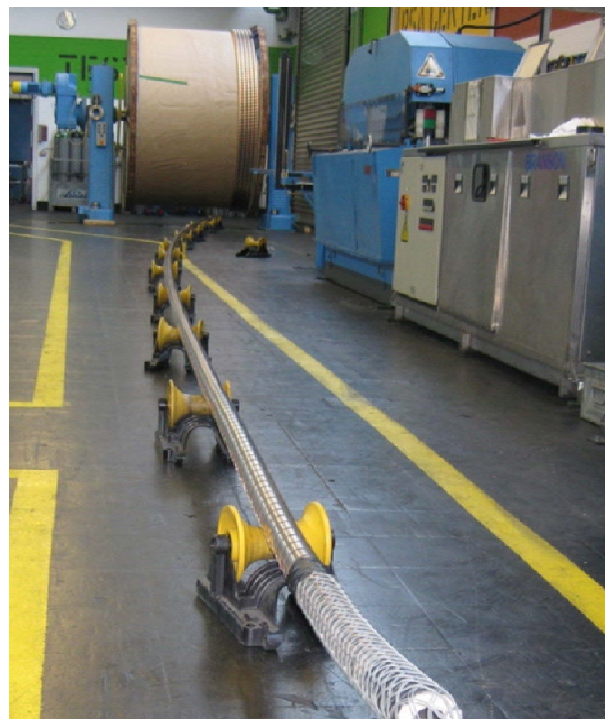
Figure 3 Bending test of pre-prototype HTS cable
