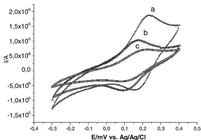
Fig. 1. Cyclic voltammogram of poly(1-vinylimidazole)<sub>12</sub>-[Os(4,4'-dimethyl-2,2'-dipyridyl)<sub>2</sub>Cl<sub>2</sub>]<sup>2+/+</sup> (osmium redox polymer) on graphite electrodes: a) with no enzyme, b) crosslinked with 0.4 U of PDH AM, and c) crosslinked with 0.4 U of WT P2O. Experimental conditions: 10 mV/s, 100 mM ethanolamine buffer, pH 9.4.
