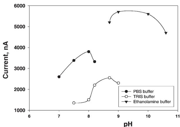
Fig. 5. Effect of different buffers and pHs on PDH from *Agaricus meleagris* based biosensors response. Experimental conditions: pH 7–8.5 phosphate buffer, pH 7.5–9 Tris-HCl, pH 8.5–10.5 ethanolamine buffer; applied potential +300 mV vs. Ag|AgCl; glucose concentration 1 mM; flow rate 1.0 mL min<sup>-1</sup>.
