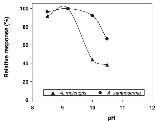
Fig. 4. Effect of pH on the response of PDH based biosensors. Experimental conditions: in ethanolamine buffer (0.1 M), applied potential +300 mV vs. Ag|AgCl; glucose 1 mM; flow rate 1.0 mL min<sup>-1</sup>.
