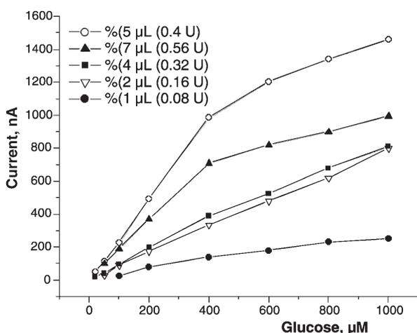
Fig. 6. Effect of amount of WT P2O on the electrode response. Experimental conditions: in ethanolamine buffer (0.1 M, pH 10.5), +300 mV vs. Ag|AgCl.
