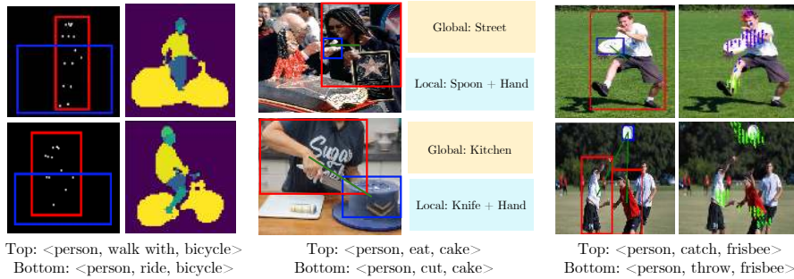
Fig. 1: (Left): Interactions with similar spatial layouts can be resolved through fine-grained spatial information . (Centre): Global and local context encode the scene and other local objects to provide strong clues for the interaction taking place; (Right): Plausible motion estimation distinguishes between interactions for which dynamics play an important role.
