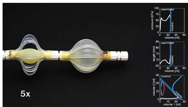
Movie S4. Inflation of a combined soft actuator—sudden increase in length. Inflation of a combined soft actuator consisting of two interconnected fluidic segments, characterized by (L_{braid}, L_{tube}) = (48, 30) and (50, 20) mm. In the experiment, we inflated the segment with water at a rate of 20 mL/min. At v = 26 ml an instability at constant volume is triggered, causing a sudden increase in length of 10 mm, which corresponds to an increase of 11%.
