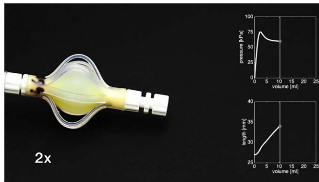
Movie S2. Inflation of a fluidic segment. Inflation of a single fluidic segment characterized by L_{braid} = 46 and L_{tube} = 20 mm. In the experiment, we inflated the segment with water at a rate of 60 mL/min.
