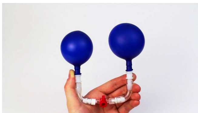
Movie S1. Two-balloon experiment. (i) Two identical balloons, inflated to different diameters, are connected to freely exchange air. Surprisingly, instead of the balloons becoming equal in size, for most cases the smaller balloon becomes even smaller and the balloon with the larger diameter further increases in volume. This unexpected behavior is the result of the nonlinear relation between the balloons' pressure and volume. (ii) By changing the initial volume of the two balloons, it is also possible to realize a system in which the balloons become equal in size when connected.
