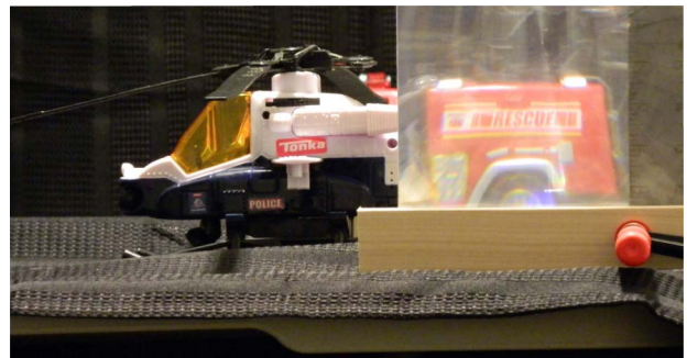
Fig. 8. Viewing along the optical axis, we see the truck appearing in the place of the tail of the helicopter. The observation was done with a 21 \times magnification camera at 6.4 m from the first lens.
