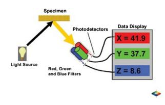
Figure 12. Illustration of a tristimulus colorimeter. Image courtesy of HunterLab.
