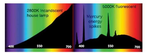
**Figure 7.** Examples of spectral power distribution from an incandescent light bulb (left) and fluorescent bulb (right) (https://en.wikipedia.org/wiki/Spectral\_power\_distribution#/media/File:Spectral\_Power\_Distributions.png; http://creativecommons.org/licenses/by-sa/3.0/deed.en).
