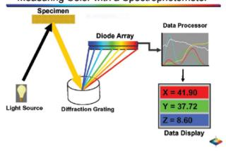
**Figure 13.** Illustration of measuring color with a spectrophotometer equipped with a photo diode array. Image courtesy of HunterLab.
