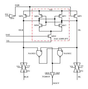
Figure 7. Read drive circuit.
