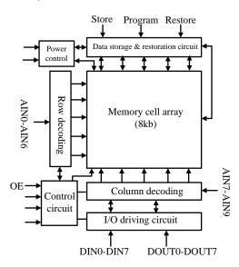
Figure 1. nvSRAM system structure.
