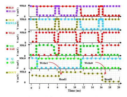
Figure 19. Simulation results for reading and writing speed.
