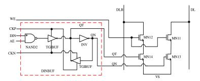
Figure 8. Write driver circuit.
