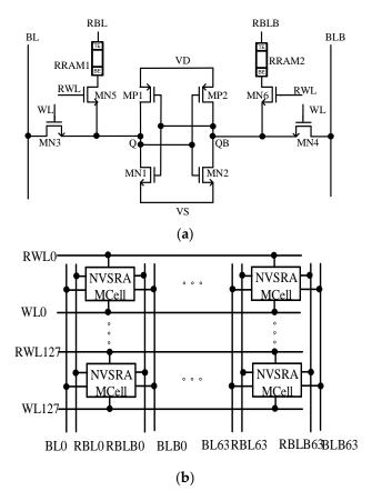
**Figure 2.** (a) 8T2R nvSRAM memory cell, (b)  $128 \times 64$  array.
