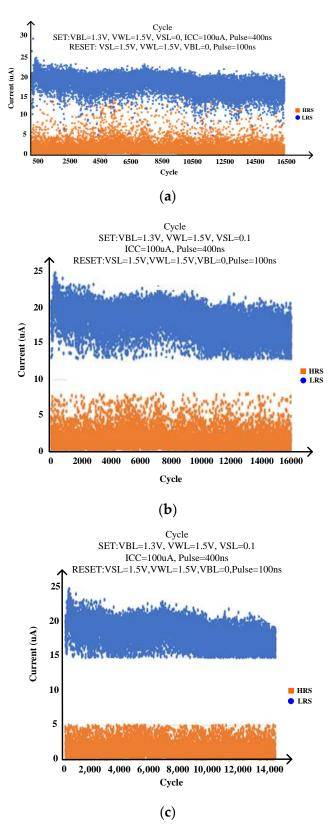
**Figure 14.** Pulse test results for 1T1R RRAM: (**a**) original data; (**b**) the data after removing the data of high-resistance current greater than 8  $\mu$ A and low-resistance current lower than 15  $\mu$ A; (**c**) data with high-resistance current greater than 5  $\mu$ A and low-resistance current lower than 13  $\mu$ A after data removal.
