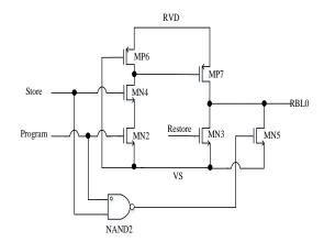
Figure 9. RRAM read/write drive circuit.
