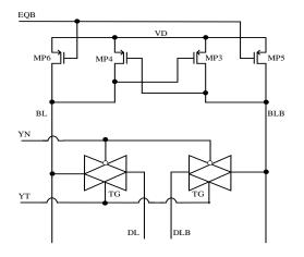
Figure 6. Column decoding circuit.
