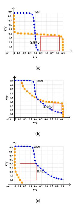
Figure 17. Noise margin: (a) static noise margin; (b) read noise margin; (c) write noise margin.
