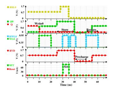
Figure 18. Simulation results for data storage and restoration circuit.
