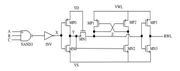
Figure 10. RWL driving circuit.
