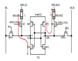
Figure 4. Data restoration operation.
