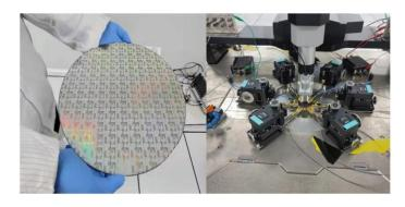
Figure 12. Die of nvSRAM and test environment.
