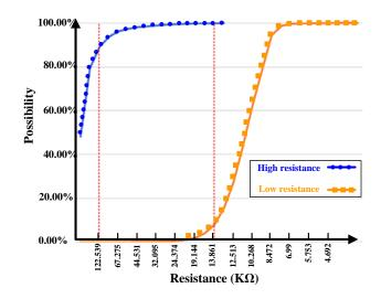
Figure 15. Resistance distribution diagram of RRAM.
