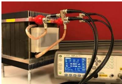
FIGURE 17. The test setup for leakage inductance measurement.
