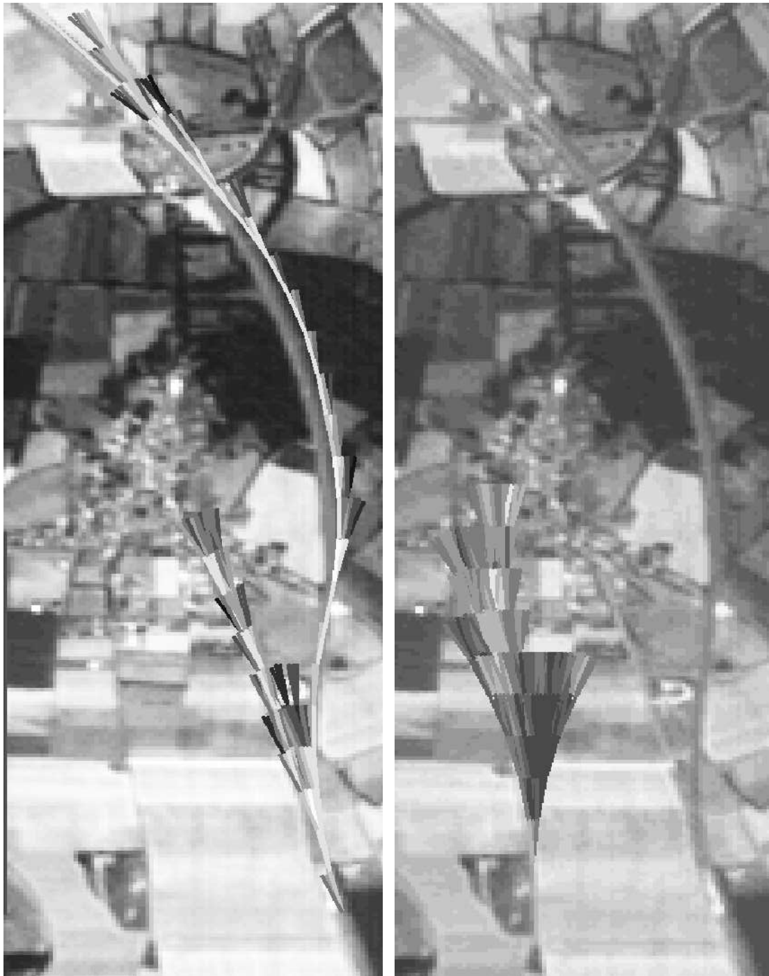
Figure 8: Left: Output of the tracking algorithm showing the arcs investigated by the algorithm in colors proportional to the likelihood ratios. Right: The tracking was initiated on a small road and is permanently stalled.
