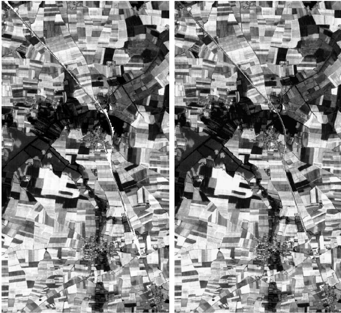
Figure 10: Left: Tracking results on a SPOT image from La Rochelle, France. The arcs selected by the algorithm are shown in white. Right: Estimate of the road
