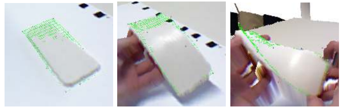
Fig. 7: The tracking sequence from real input data. The images show a colored 3D mesh, based directly on the Kinect input data along with the deformation function (green grid) roughly approximating the object surface.
