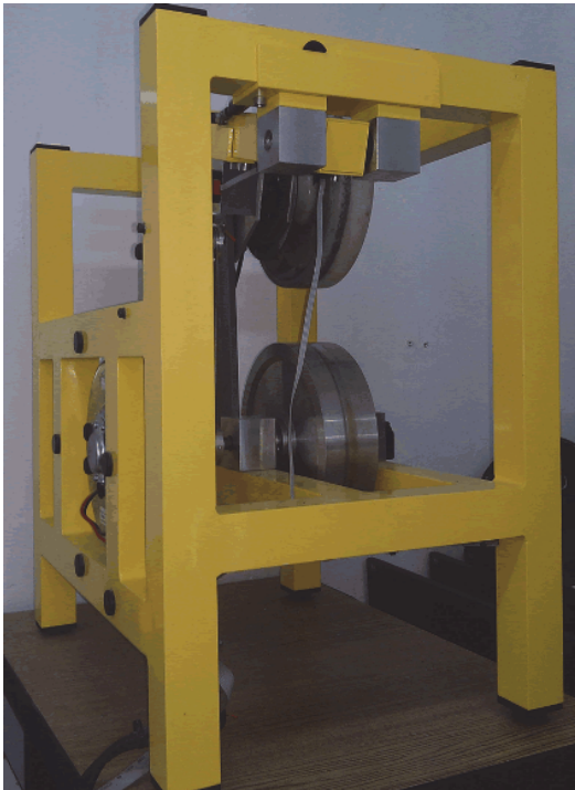
Figure 4. The ABS laboratory setup [11]. Source: Inteco Manual [11].
