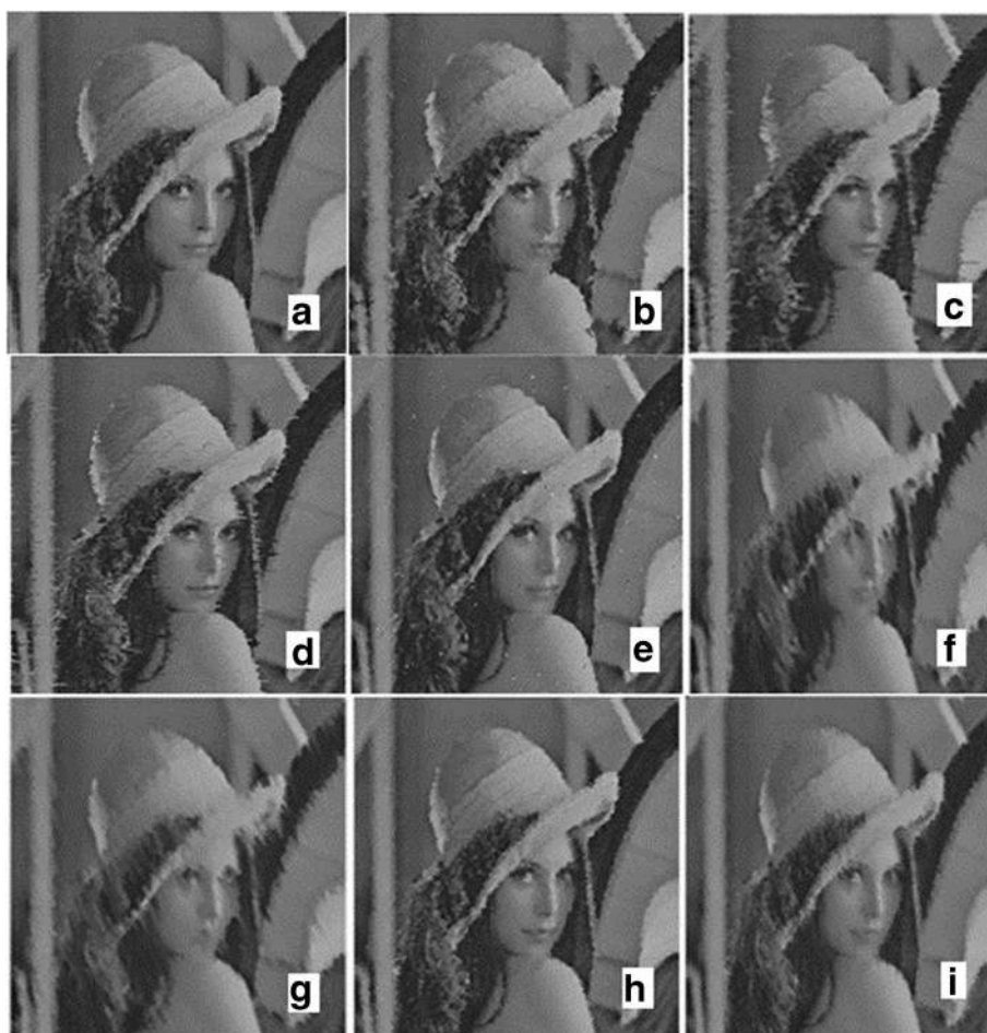
Fig. 10 Performance of various algorithms corrupted by 90% salt and pepper noise on Lena image a DBIDWIF, b AMF ( W_{max} = 39 ), c DBA, d IDBA, e NAFSM, f MDBUTMF, g MDBUTMF-GM, h ACBSA, and i AWMF ( W_{MAX} = 39 )
