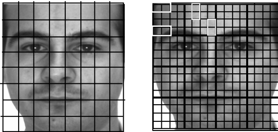
Fig. 3 (a) Left image shows non-overlapping modules, each of size 8×8 pixels (b) The right image shows the creation of CHBs and CVBs, (white rectangular boxes) from two small 4×4 regions. The smaller blocks are 4×4 pixel regions and the thicker, larger blocks are the neighborhoods
