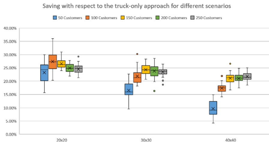
Figure 21: Distribution of the saving obtained by serving the customers using a mixed truck/drone approach compared to using a truck-only approach (SVRP) for different scenarios, when considering 15 minutes of total endurance time. The average saving for each scenario is marked with a cross.
