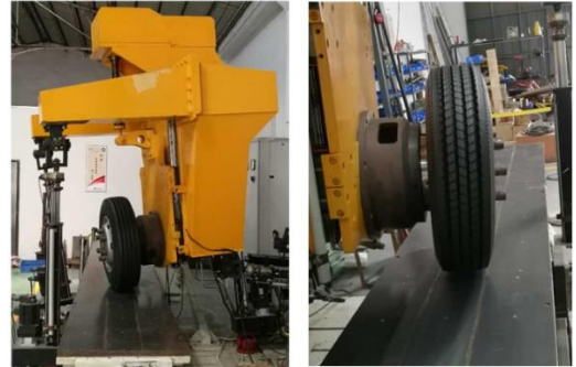
Figure 1 Experimental setup of the tire mechanical characteristics tests.
