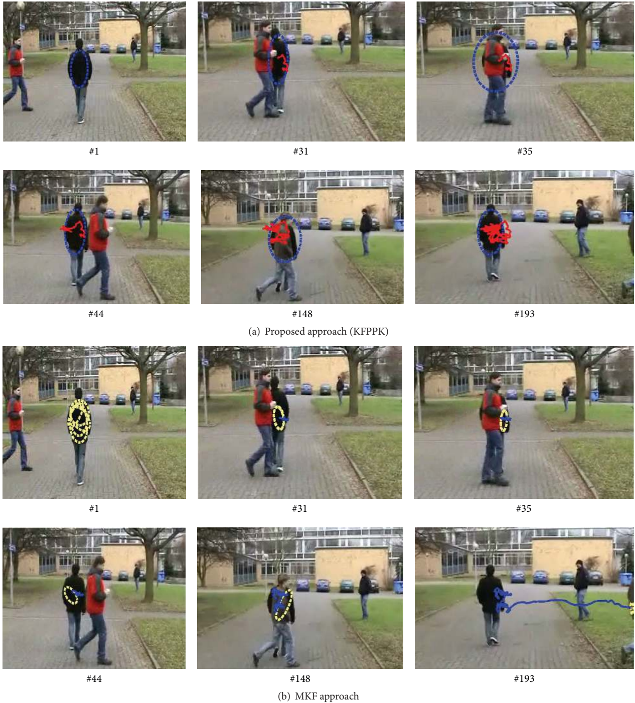
FIGURE 4: Tracking results of the occlusion sequence by different tracking algorithms. Frames 1, 31, 35, 44, 148, and 193 are displayed.
