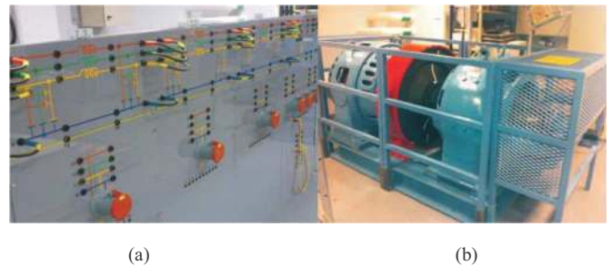
Fig. 10. Photograph of the laboratory setup. (a) Analog transmission-line model. (b) Generator system.
