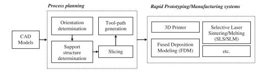
Fig. 1. Process planning for RP/M systems.
