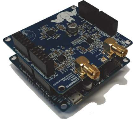
FIGURE 4: YetiMote WSN node used for testing the adaptive scheduler.
