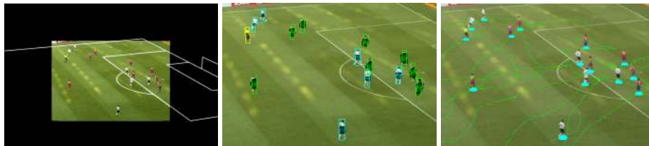
Fig. 7. Camera estimation (left), player observation (center) and trajectory generation (right)
