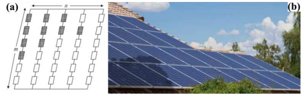
Fig. 2. (a) The schematic model of a PV array under PSC and (b) real PSC in a PV array.
