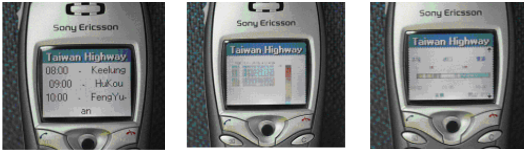
Figure 9: Delivering ITWS traveler information to cellular phone display
