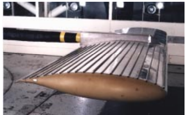
Figure 5c. GA(W)-1 model with Small Hemispherical Bumps and high density distribution (HDSB).
