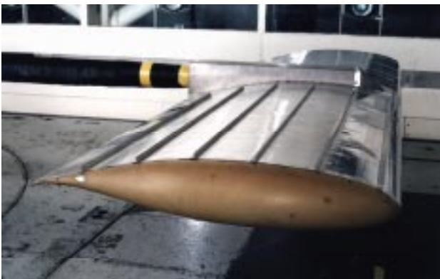
Figure 4c. GA(W)-1 model with Large Vertical Plates and low density distribution (LDLP).
