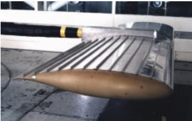
Figure 4b. GA(W)-1 model with Large Vertical Plates and medium density distribution (MDLP).
