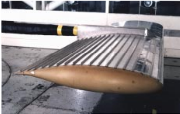
Figure 4a. GA(W)-1 model with Large Vertical Plates and high density distribution (HDLP).
