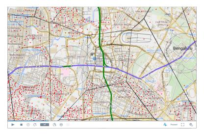
Figure 2: AnyLogic simulator showing the OSM network and Voronoi regions. Purple and green lines are the metro routes, and red dots represent centroids of EBs, which are potential origins/destinations. The circles indicate regions which are within 500 m.
