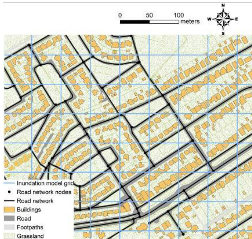
Figure 5 A detail showing the road network, building locations and inundation model raster grid
