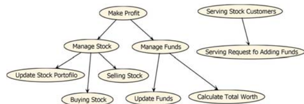
Figure 1. Example of a goal overview diagram for a stock trading management system
