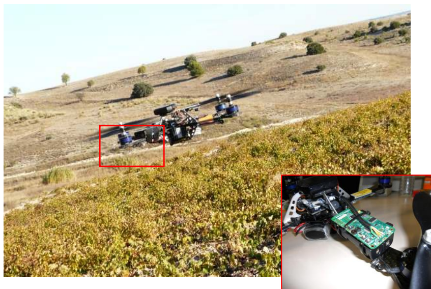
Figure 8. Quadrotor on-board mass distribution.
