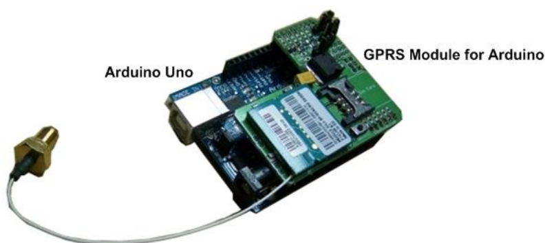
Figure 9. Arduino system employed for communication with the base station, likewise for message delivery.
