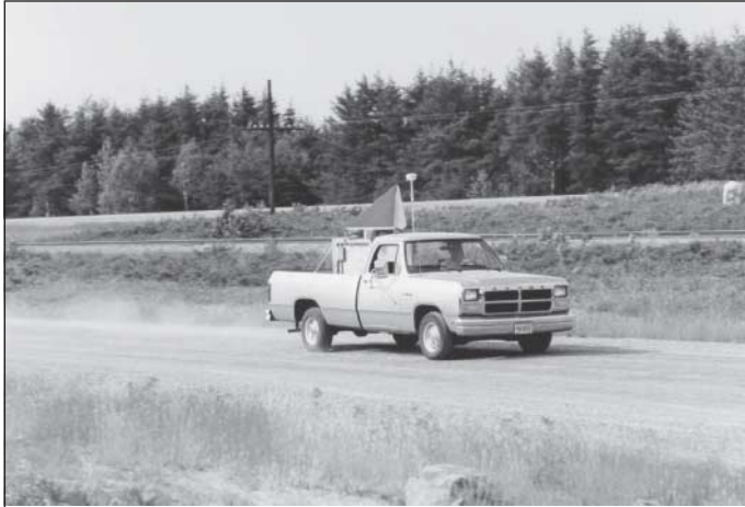
Figure 7. Pickup truck as a GMT on dirt road, with corner reflector and DGPS antenna.
