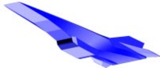
Figure 2. Hyper-X Research Vehicle with Airframe-Integrated, Dual Mode Ramjet/Scramjet Propulsion
