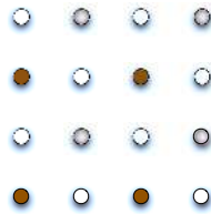
Figure 4.4: An illustration of three (self-similar) probing grids. We choose \mathcal{L}_j = (1+i)^j \mathbb{Z}[i] ( j = 0, 1, 2 ) and \mathcal{R} = [0, 3] \times [0, 3] . The sparsest grid consists of 4 solid points. The second sparsest grid consists of 4 solid points and 4 partially solid points.
