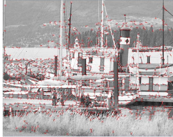
Figure 2: An example of corners detected using our algorithm
