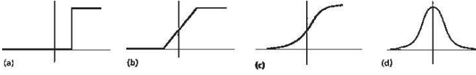
Fig. 5: Different types of activation functions: (a) threshold, (b) piecewise linear, (c) sigmoid, and (d) Gaussian.
