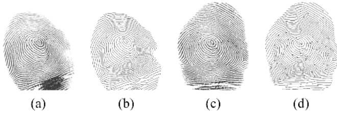
Fig. 6. Experimental results on two fingerprints in NIST 24. The images have been scaled for view: (a) original image, (b) thinned image of (a), (c) original image, and (d) enhanced image of (c). The similarity of these two fingerprints is 0.62272.
