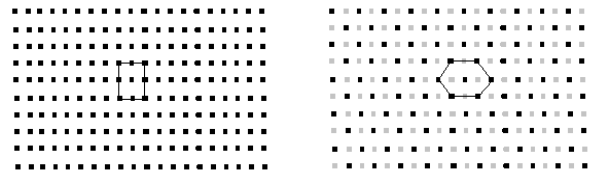
Fig.4. (a) Rectangular grid and (b) Simulated hexagonal grid obtained using alternate pixel suppression
